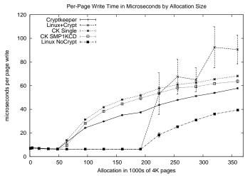
Fig. 3. Write performance comparison of five kernels as allocation sizes increase.
