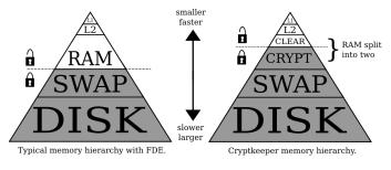
Fig. 2. Comparison of traditional memory hierarchy with CK. Levels below the dotted line are encrypted, levels above are unencrypted.
