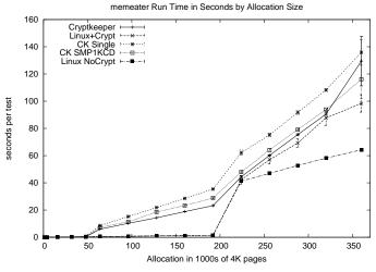
Fig. 5. Wall clock time comparison of five kernels as allocation sizes increase.
