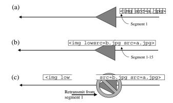
Figure 5: Failure recovery using Semantic Segmentation – (a) one byte segments arrive at adaptor, (b) segment combination and adaptation occurs, (c) failure requires segment recovery.
