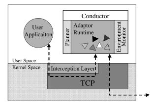
Figure 1: The Conductor architecture deployed on a node.
