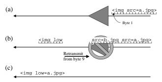
Figure 4: Failure recovery using a byte-count – (a) data arrives at adaptor, (b) failure and retransmission occur, (c) retransmission produces an undesirable result.
