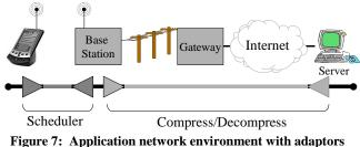
Figure 7: Application network environment with adaptors deployed.
