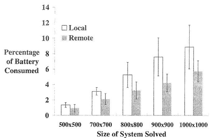
Figure 3: Power savings for remote execution of Gaussian solution of a system of linear algebraic equations
