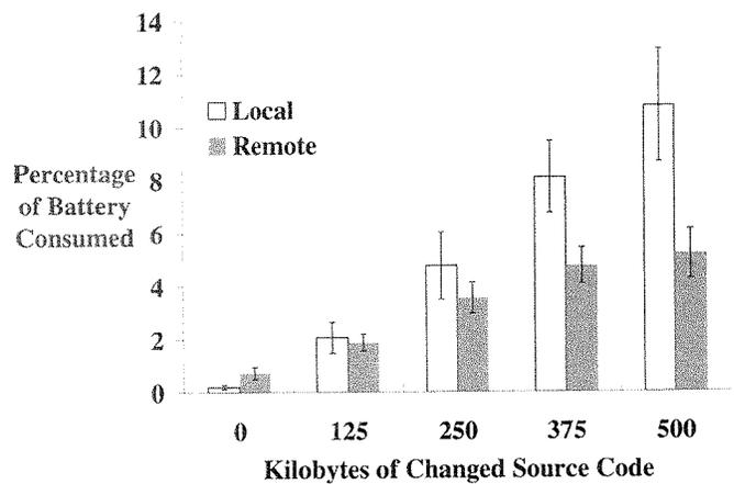
Figure 1: Power savings for remote execution of a compilation
