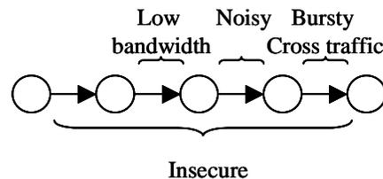
Figure 2. A data path with multiple problems
