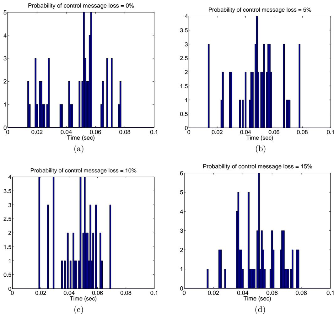
Figure 4: Settling time distributions for routing change recovery
