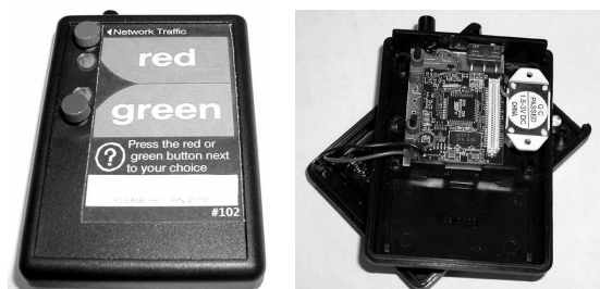
Figure 1: External and internal views of a mote-based voting device.
