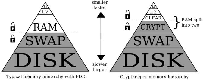
Fig. 2. Comparison of traditional memory hierarchy with CK. Levels below the dotted line are encrypted, levels above are unencrypted.
